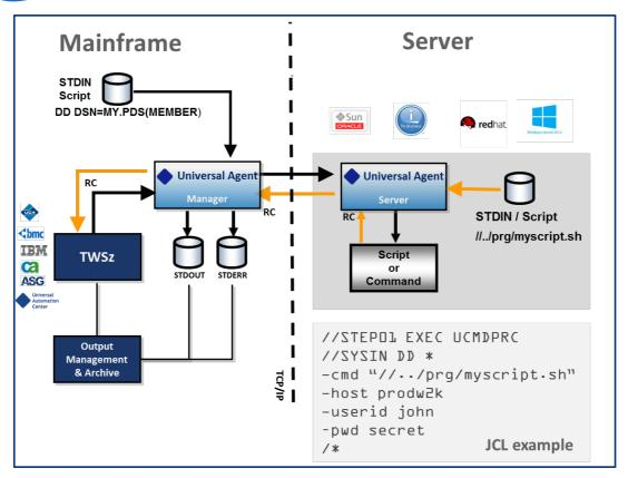
Figure 3: Triggering a UNIX script from the mainframe via Universal Agent
